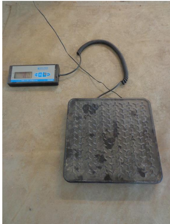
Figure 9. Scale with maximum measurement of 136 kg +/- 0.23 kg
