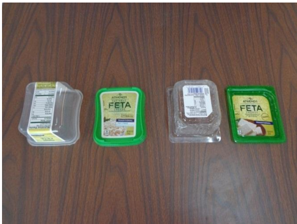
Figure 14. Feta containers from left to right: PP container, PP lid, PVC container, PVC lid
