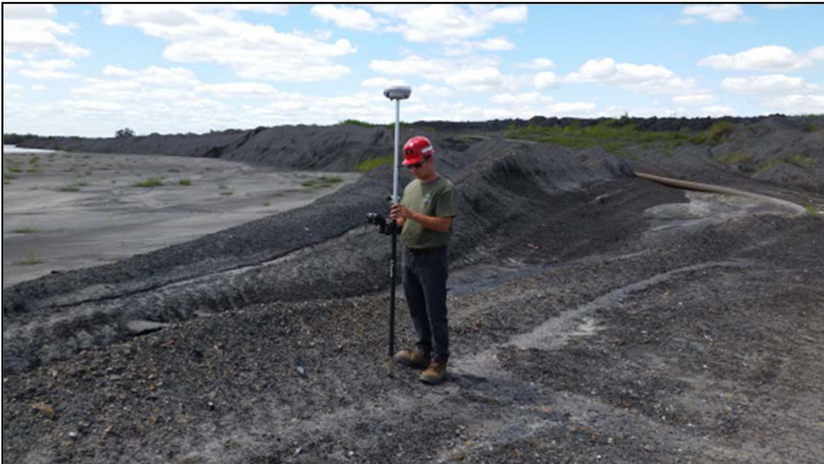
Figure 4: Intern using a Trimble R6 GPS to take elevation points of Old Ed Carbon Recovery Mine.
