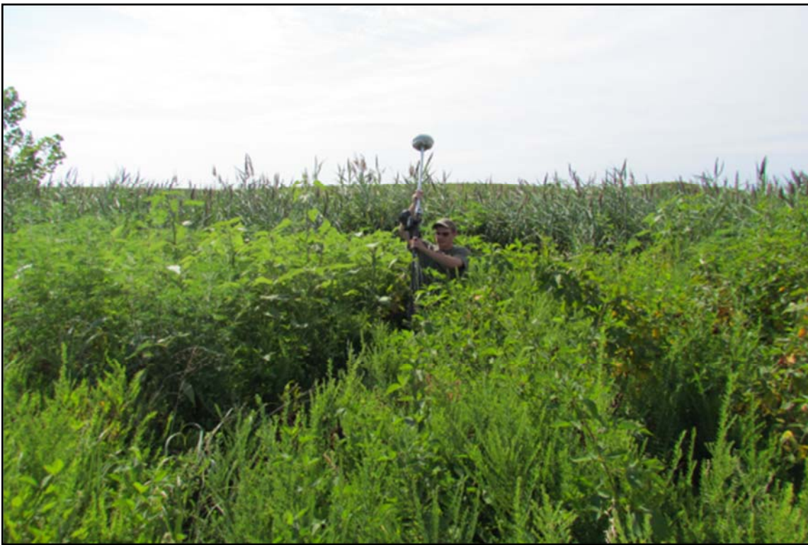
Figure 6: Intern using a Trimble R6 GNSS GPS to map areas of Phragmites australis .
