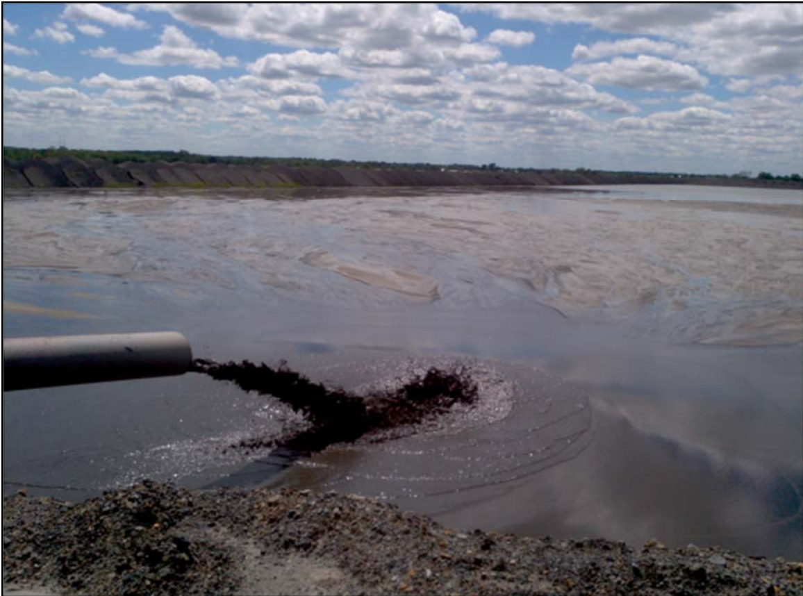
Figure 5: Slurry is being pumped into a slurry pond at Red Hawk Mine.
